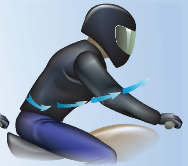
Phase 3: let air escape by using front zipper only. Repeat steps to stay cool until sleeves need more water. Add water and repeat.
