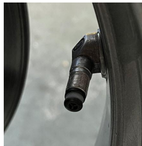
Inner valve stem backed out.
