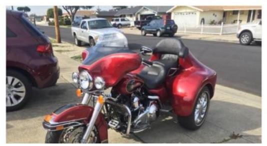
2007 Harley Classic with DFT trike kit installed. Kit uses independent rear suspension like a corvette and custom body work with large storage area (trunk). This trike is also equipped with an electronic hand shifter and reverse gear. Foot shifter is still working as well. Has less than 3,200 miles. \$35K invested. **Asking only \$21,000.**
