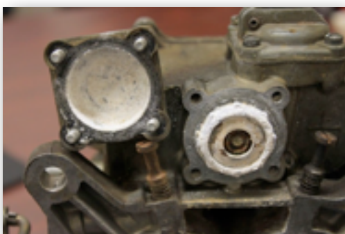
Reported E15 damage to a carburetor
